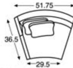
LTD7460-41 LAF CHAIR Overall: W51.75 D36.5 H38.5 Inside: W32.5 D18 H19 Seat Height: 19.5 Arm Height: 16.5
